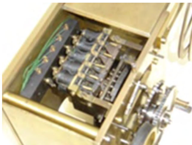
The five electromagnets of the printer receiver
